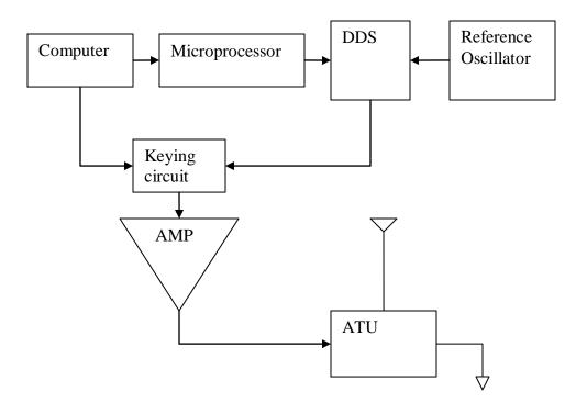
Figure 1. Experimental 504-509 kHz transmitter system block diagram.
