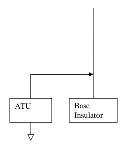
Figure 3. Proposed monopole aerial comprising a guyed steel tower up to 25 metres high resting on a ceramic base insulator. The earth connection will be via 12 equally spaced radials 30 metres long on the ground surface. The ATU is fed with 50 Ohm coaxial cable from the transmitter.
