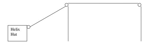
Figure 2. 100m wire aerial at 10 metres average height. The wire slopes up over a length of 30 metres. The horizontal portion is suspended from insulators from 10 metre masts
